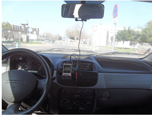
(c) Acquiring in-vehicle speech samples in hands-free mode with an external microphone.
